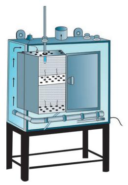
Fig. 5.1: Hot air oven
