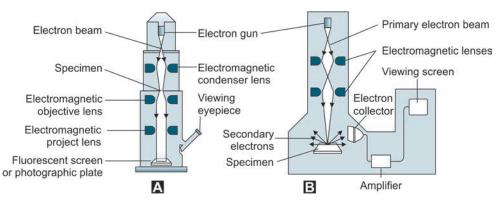
Fig. 2.3: (A) Transmission and (B) scanning electron microscopy. The illustrations show the pathways of electron beams used to create images of the specimens
