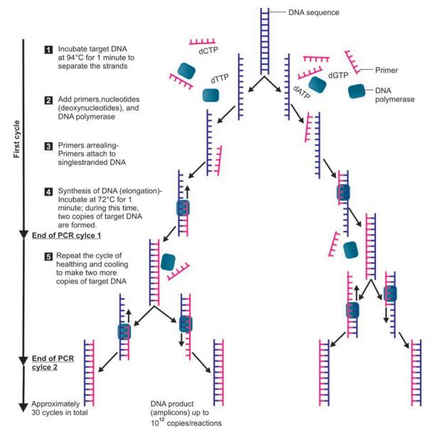
Fig. 10.19: Polymerase chain reaction
