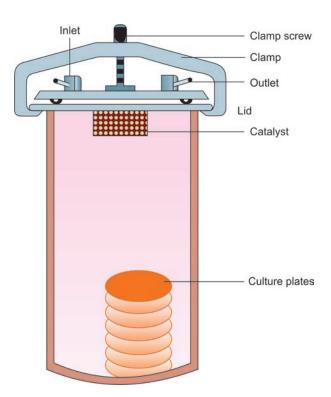
Fig. 7.2: McIntosh and Filde's anaerobic jar
