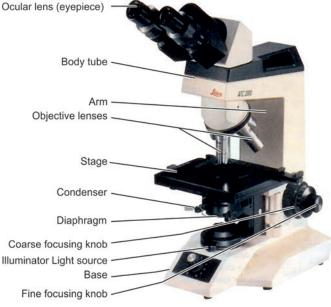
Fig. 2.1: Principal parts of compound light microscope
